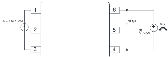
Figure 19 : UVLO Test Circuit
